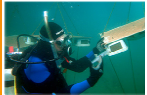
Pre-settlement, larval bryozoans (a common fouling organism) are injected into a chamber to test for the effects of heavy metals (copper) influencing marine communities in ports and harbours.
